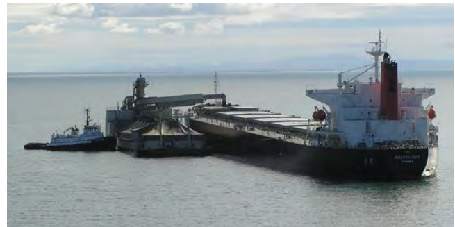
Tug and concentrate barge unloading to an ocean-going vessel
