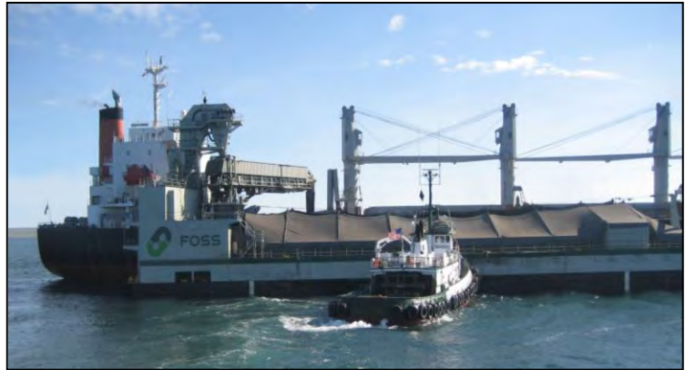
Lightering of concentrates to the ocean transport vessel
